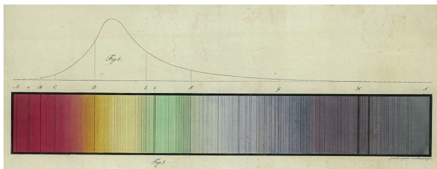
Figure 1: Sun spectrum with the Fraunhofer lines (left). Photo: Joseph Fraunhofer, 1814. Deutsches Museum, München, Archiv, BN43952, CC BY-SA4.0. Right: Photo of Fraunhofer's prism spectrograph, located at the Deutsches Museum. Photo: Birgitta Schultze-Bernhardt
